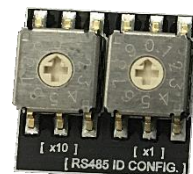
Picture 1. Rotary Switch
